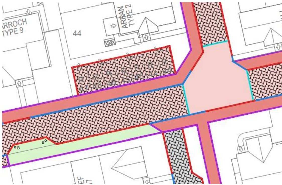
Extract above from superseded drawing (document 46) showing allocated EV charging points as prospectively adoptable (red).
