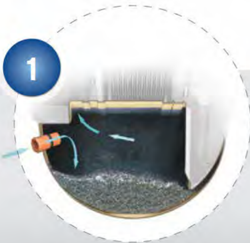
1 PRIMARY SETTLEMENT TANK Wastewater and sewage flows into the primary settlement tank where the large solids are retained for future removal.
