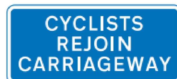
Figure 11-18 Diagram 956 (S3-2-29) Route for use by pedal cycles and pedestrians only
