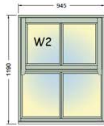
Window Elevation W2 @ 1-25
