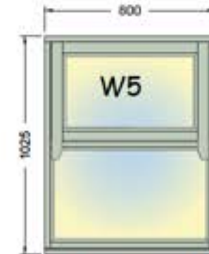
Window Elevation W5 @ 1-25
