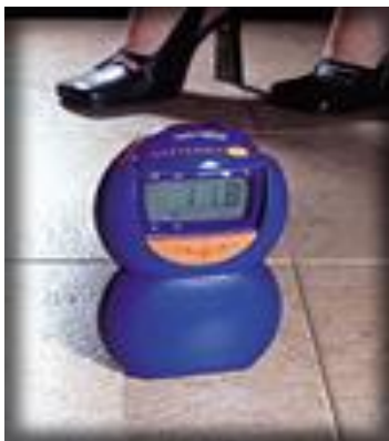
Typical surface roughness measuring instrument, the “Surtronic Duo”. Further information on instrumentation available at: Assessing the slip resistance of flooring (hse.gov.uk)
