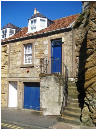
Traditional design of fishermen's houses- with ground floor workshop/sail loft and later dormer with gantry and hoist to attic floor sail store. Example below with fore-stair.
