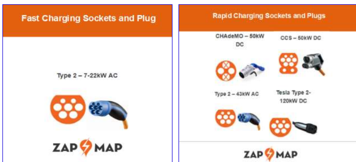
Figure C-2. Type 2 Socket and Plugs for Trickle / Fast and Rapid Charging in the UK (Source: Zap-Map, final figure to be improved)
