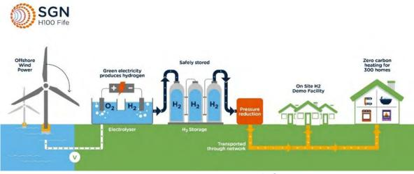
Figure 7: H100 System Diagram – Copyright © SGN
