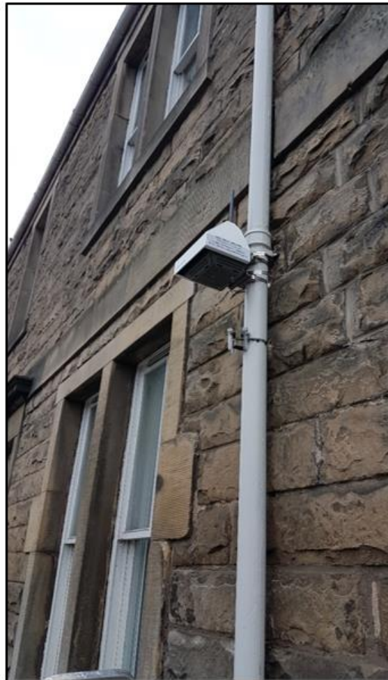
Appin Crescent West AQMesh sensor (co-located with triplicate diffusion tubes Appin Crescent 6A,B & C)
